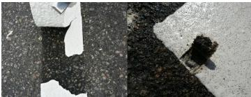
HEAT MUST BE DISTRIBUTED EVENLY. MELTMARK MUST MELT AND HEAT MUST ALSO REACH THE UNDERLYING SURFACE.
