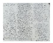
Two pictures from left shows correcty applied MeltMark. Pictures taken after some seconds of cooling. MeltMark has fully anchored to underlying surface and enough heat has reached the underlying surface. This test method destroys the marking and is only used here for clarifying importance of correct heating.
