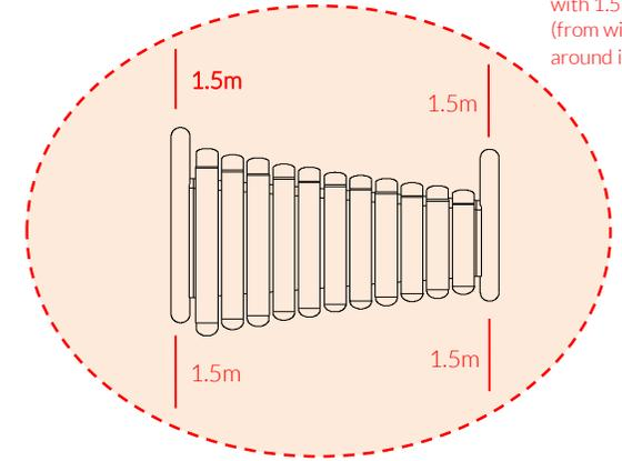
Install Instrument with 1.5m free space (from widest point) around it.
